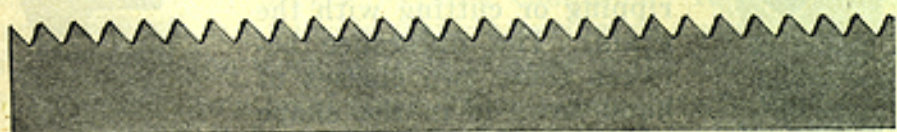
Section of 8 point saw for cross-cutting
