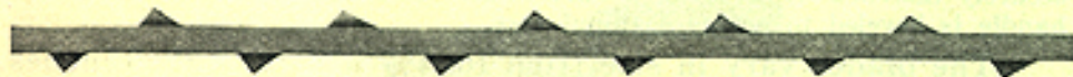
Fig. 3—Looking from the back of a saw. This shows how the teeth, when set, extend beyond the edge of the blade
