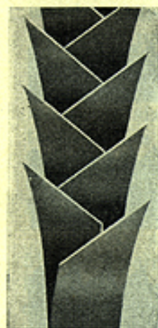
Tooth edge of saw for cross-cutting
